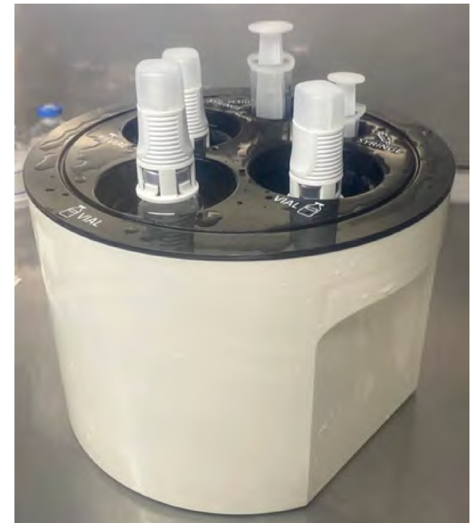
Fig.2 Chilling block used to keep product temperature low
