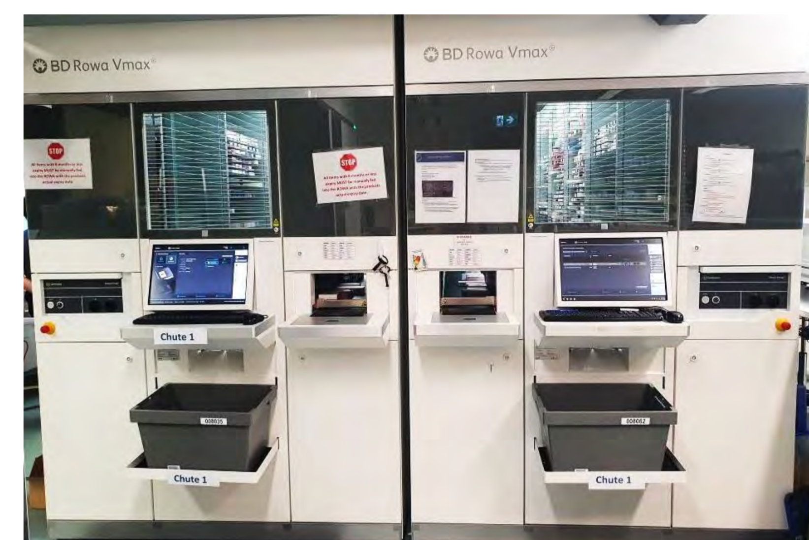
Figure 1: Automated dispensing robot at the Lyell McEwin Hospital pharmacy in South Australia
